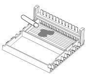
4.2.3 Hold the two sides of comb and pull out slowly after the gel solidified. The hole of gel should be ordered and without damage.
