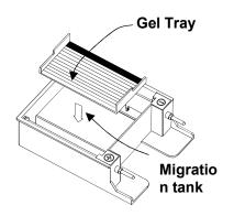
4.3.2 Pour buffer solution to a level of about 3mm above the surface of the gel, 250-300ml of buffer is required.
