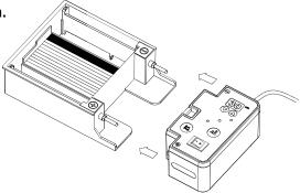
4.2.3 Pour the gel into gel maker stand with the tray and the height should around 4mm and each tray need about 25ml gel.
