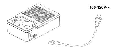
1.3.3 When the input voltage is AC220V, please use adaptor to transform, please connect both instrument and adaptor as below
